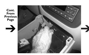
**STEP 7:** Pull up and remove the cup holders.
